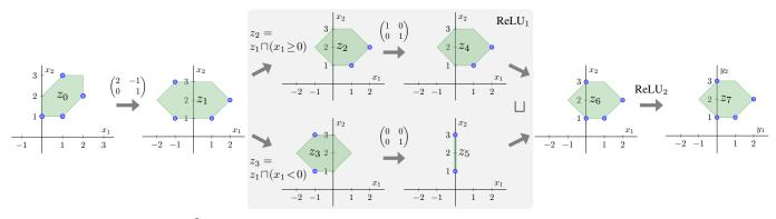
Fig. 7: Illustration of how  $AI^2$  overapproximates neural network states. Blue circles show the concrete values, while green zonotopes show the abstract elements. The gray box shows the steps in one application of the ReLU transformer (ReLU<sub>1</sub>).
