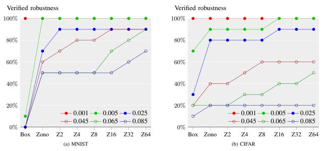
Fig. 10: Verified properties as a function of the abstract domain used by  $AI^2$  for the  $9 \times 200$  network. Each point represents the fraction of robustness properties for a given bound (as specified in the legend) verified by a given abstract domain (x-axis).
