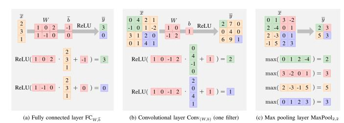
Fig. 4: One example computation for each of the three layer types supported by AI<sup>2</sup>.
