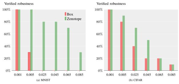
Fig. 9: Verified properties by AI<sup>2</sup> on the MNIST and CIFAR convolutional networks for each bound  $\delta \in \Delta$  (x-axis).
